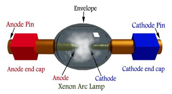
When in the excited atoms, the electrons return from its higher energy level to its previous energy state, the extra energy is released as a photon. The wavelength of energy emitted through photons is within visual range. The color of the light of xenon arc light is like daylight. Due to the electrostatic attraction of anode or positive electrodes, the free electrons originated due to the ionization process ultimately comes to the anode and returns to the source.
